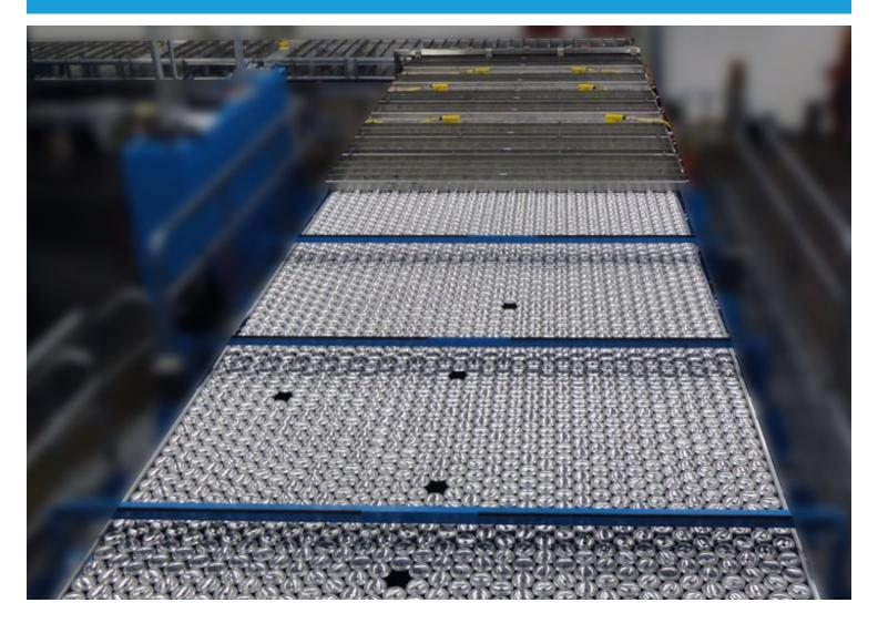
BW Integrated Systems' patented Isometric Air Conveyor Washer Infeed guarantees gently-packed, inverted cans at the infeed of the can washer. This technology has been a game-changer for troublesome washer infeeds and is revolutionizing this area of can lines by eliminating damaged cans, reducing scrap and increasing line efficiencies.
